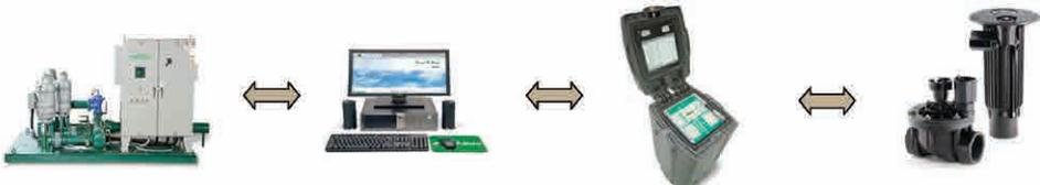
A diagram illustrating the integration of various irrigation components. From left to right: a control panel with multiple valves, a desktop computer with a monitor and keyboard, a handheld handheld device with a screen, and a valve assembly with a solenoid. Double-headed arrows connect each component to the next, indicating their interconnected nature.
